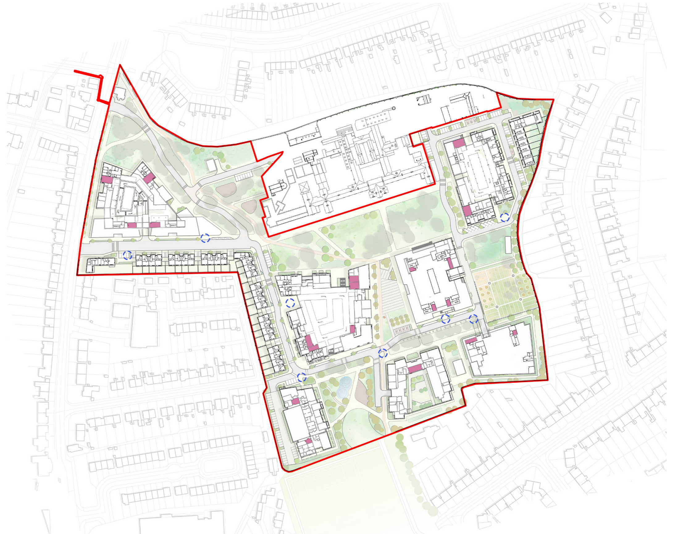
Figure 15 - Ground floor plan with waste room locations shown in magenta and waste staging areas circled.
